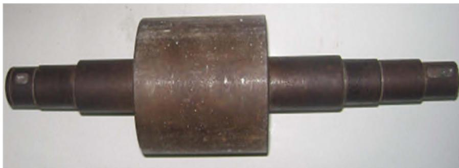
**Fig - I.8** - Rotor massif
