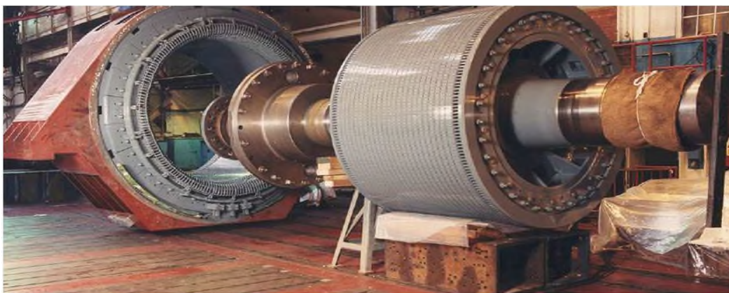
Figure I.1 : Machine asynchrone de 4.7 MW, 45tr/mn [3]
