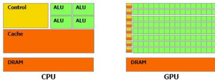
Figure III.3 Architecture CPU et GPU [NVIDIA].
