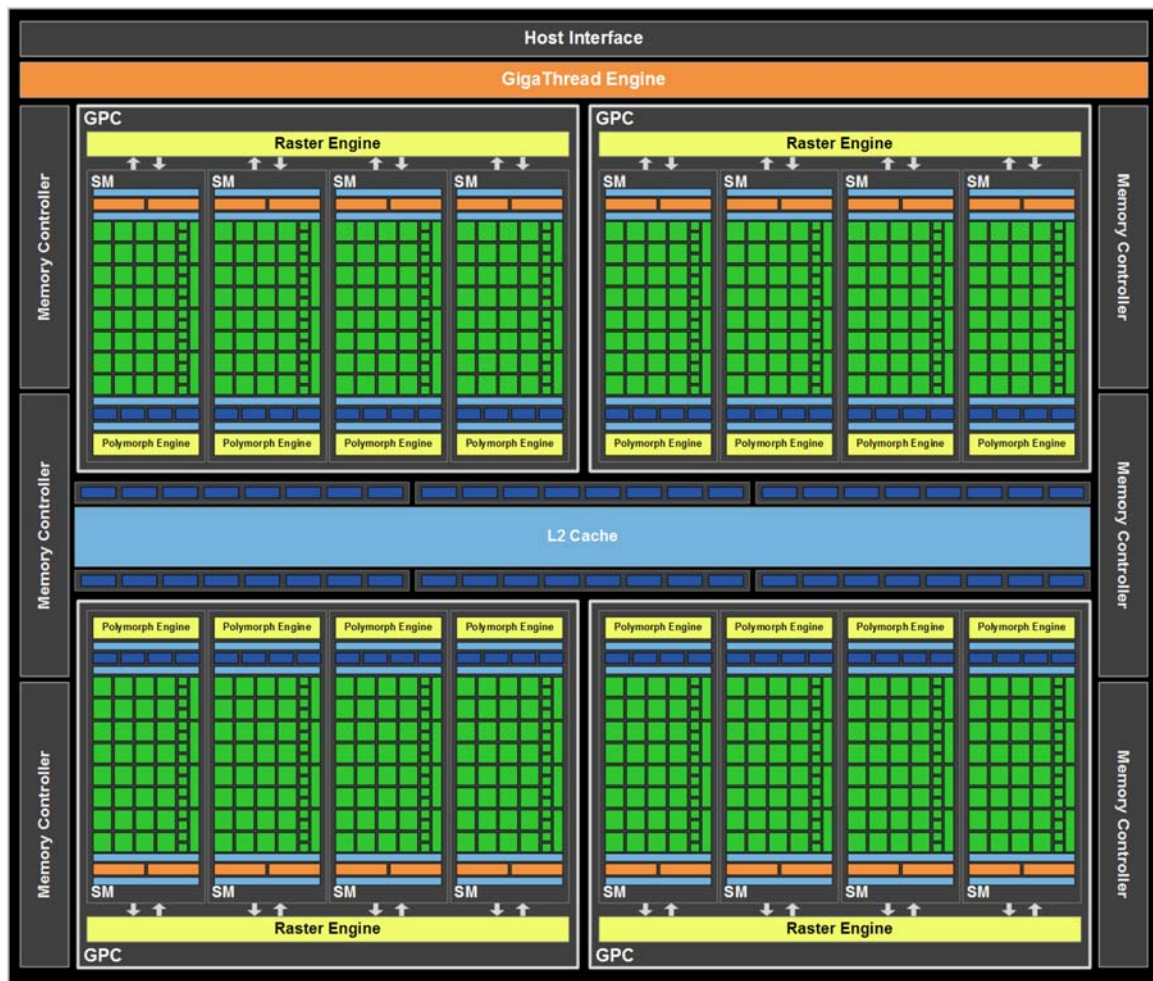
Figure III.6 : Architecture Fermi [Nvidia]
